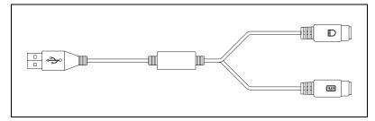
Figure 4-1. Y-Splitter Cable
